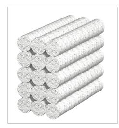
The noise limit barrier is used to reduce the transmission of airborne noise, e.g. when the trunking system is run through a wall between two offices. The noise limit barrier is made of rock wool, which, when delivered, has a diameter of approx. 50 mm and a length of approx. 300 mm. The material need not be greatly compressed during installation.
